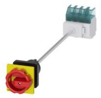
SENTRON, Switch disconnector 3LD, emergency switching-off switch, 4- pole, lu: 32 A, operating power / at AC-23 A 400 V: 11.5 kW, floor mounting with door coupling, rotary operating mechanism, Red / yellow, central mounting 22.5 mm of the handle
