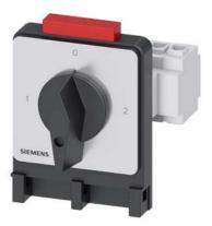
SENTRON, Switch disconnector 3LD, change-over switch, 4-pole, lu: 32 A, Operating power / at AC-23 A at 400 V: 11.5 kW, front-mounted, knob-operated mechanism, black, 4-hole mounting of the handle, in neutral position can be locked
