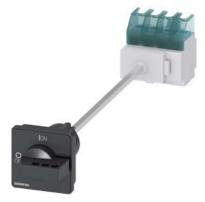
SENTRON, switch disconnector 3LD, main switch, 4-pole, lu: 32 A, operating power / at AC-23 A at 400 V: 11.5 kW, floor mounting with door coupling, defeatable knob-operated mechanism, black, 4-hole mounting of the handle
