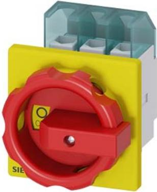
SETRON, Switch disconnecter 3LD, emergency switching-off switch, 3- pole, Iu: 32 A, operating power / at AC-23 A 400 V: 11.5 kW, front-mounted, rotary operating mechanism, Red / yellow, 4-hole mounting of the handle
