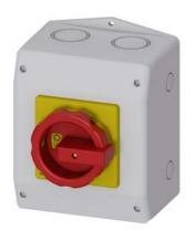
SENTRON, Switch disconnector 3LD, emergency switching-off switch, 6- pole, lu: 25 A, operating power / at AC-23 A 400 V: 9.5 kW, Molded plastic encapsulation for metric cable gland, 1 NC, 1 NO, rotary operating mechanism, red/yellow
