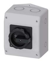
SENTRON, Switch disconnector 3LD, main switch, 6-pole, lu: 25 A, Operating power / at AC-23 A at 400 V: 9.5 kW, molded-plastic encapsulation for metric screw connection, 1 NC, 1 NO, rotary operating mechanism, black
