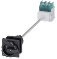
SENTRON, Switch disconnector 3LD, main switch, 3-pole, lu: 25 A, Operating power / at AC-23 A at 400 V: 9.5 kW, floor mounting with door coupling, rotary operating mechanism, black, central mounting 22.5 mm of the handle
