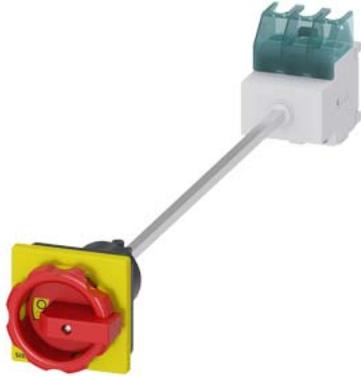
SETRON, Switch disconnecter 3LD, emergency switching-off switch, 3- pole, Iu: 25 A, operating power / at AC-23 A 400 V: 9.5 kW, floor mounting with door coupling, rotary operating mechanism, Red / yellow, 4-hole mounting of the handle
