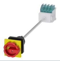
SENTRON, Switch disconnector 3LD, emergency switching-off switch, 3- pole, lu: 16 A, operating power / at AC-23 A 400 V: 7.5 kW, floor mounting with door coupling, rotary operating mechanism, Red / yellow, central mounting 22.5 mm of the handle
