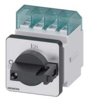
SENTRON, Switch disconnector 3LD, main switch, 3-pole, lu: 16 A, Operating power / at AC-23 A at 400 V: 7.5 kW, front-mounted, knob-operated mechanism, black, 4-hole mounting of the handle
