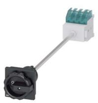
SENTRON, Switch disconnector 3LD, main switch, 3-pole, Iu: 16 A, Operating power / at AC-23 A at 400 V: 7.5 kW, floor mounting with door coupling, rotary operating mechanism, black, 4-hole mounting of the handle
