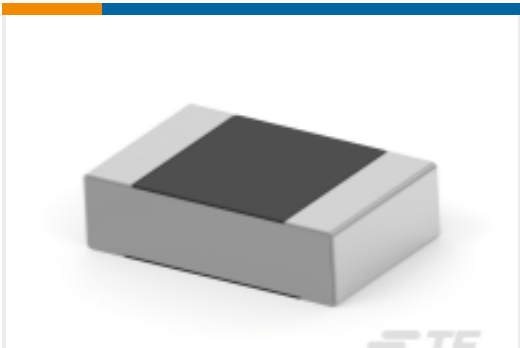
TE Part # 5-2176238-6 CPF A 0805 25K 0.1% 25PPM 5K RL
