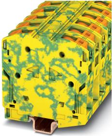
Ground modular terminal block, number of connections: 2, number of positions: 1, connection method: Power-Turn connection, 1 level, Rated cross section: 95 mm<sup>2</sup>, cross section: 25 mm<sup>2</sup> - 95 mm<sup>2</sup>, mounting type: 2.3 mm copper DIN rail, color: green-yellow
