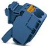
Pick-off terminal block, For use with PTPOWER 50, 95, 150, and 185 Power-Turn high-current terminal blocks, nom. voltage: 1500 V, nominal current: 57 A, connection method: Push-in connection, 1 level, Rated cross section: 10 mm<sup>2</sup>, cross section: 0.5 mm<sup>2</sup> - 16 mm<sup>2</sup>, mounting type: on base element, color: blue
