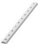
Zack Marker strip, flat, Strip, white, labeled, Printed vertically: consecutive numbers 1 ... 10, 11 ... 20, etc. up to 91 ... 100, mounting type: snap into flat marker groove, for terminal block width: 10 mm, lettering field size: 5.15 x 10 mm, Number of individual labels: 10
