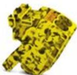
Pick-off terminal block, For use with PTPOWER 50, 95, 150, and 185 Power-Turn high-current terminal blocks, nom. voltage: 1500 V, nominal current: 57 A, connection method: Push-in connection, 1 level, Rated cross section: 10 mm<sup>2</sup>, cross section: 0.5 mm<sup>2</sup> - 16 mm<sup>2</sup>, mounting type: on base element, color: black/yellow
