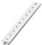
Marker for terminal blocks, Strip, white, labeled, can be labeled with: CMS-P1-PLOTTER, horizontal: L1, L2, L3, N, PE, L1, L2, L3, N, PE, mounting type: snap into tall marker groove, for terminal block width: 10.2 mm, lettering field size: 10.15 x 10.5 mm, Number of individual labels: 10
