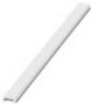
Zack Marker strip, flat, can be ordered: Strip, white, labeled according to customer specifications, mounting type: snap into flat marker groove, for terminal block width: 10 mm, lettering field size: 5.15 x 10 mm, Number of individual labels: 10
