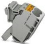
Pick-off terminal block, For use with PTPOWER 50, 95, 150, and 185 Power-Turn high-current terminal blocks, nom. voltage: 1500 V, nominal current: 57 A, connection method: Push-in connection, 1 level, Rated cross section: 10 mm<sup>2</sup>, cross section: 0.5 mm<sup>2</sup> - 16 mm<sup>2</sup>, mounting type: on base element, color: gray
