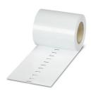
Marker for terminal blocks, Roll, white, unlabeled, can be labeled with: THERMOMARK ROLL 2.0, THERMOMARK ROLL, THERMOMARK ROLL X1, THERMOMARK ROLLMASTER 300/600, THERMOMARK X1.2, THERMOMARK S1.1, perforated, mounting type: snapped, snap into flat marker groove, for terminal block width: 10.2 mm, lettering field size: 6.35 x 10.15 mm, Number of individual labels: 10000
