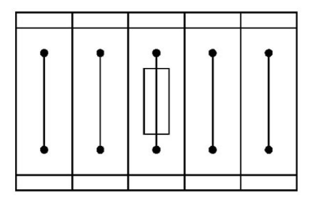
Fuse terminal block in single arrangement,
