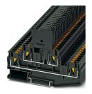
Fuse modular terminal block, fuse type: Glass / ceramics / ..., fuse type: G / 5 x 20, nom. voltage: 24 V, nominal current: 28 A, connection method: Push-in connection, 1 level, Rated cross section:  $4 \text{ mm}^2$ , cross section:  $0.2 \text{ mm}^2$ -  $6 \text{ mm}^2$ , connection method: Push-in connection, 2nd level, Rated cross section:  $4 \text{ mm}^2$ , cross section:  $0.2 \text{ mm}^2$ -  $6 \text{ mm}^2$ , mounting type: NS 35/7,5, NS 35/15, color: black
