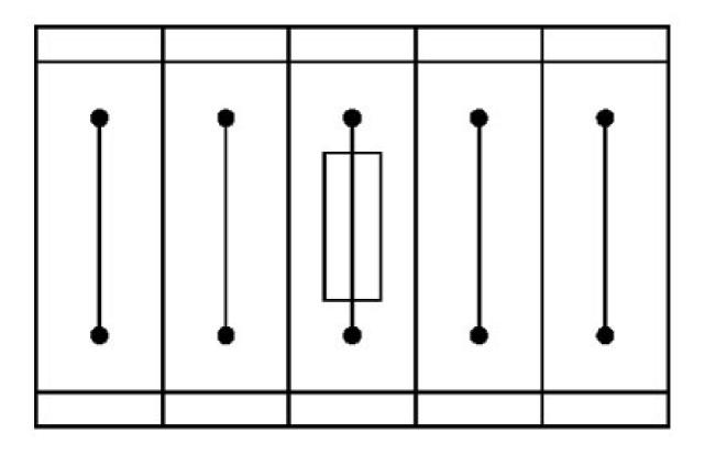
Fuse terminal block in single arrangement,
