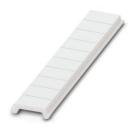
Zack Marker strip, flat, Strip, white, unlabeled, can be labeled with: PLOTMARK, CMS-P1-PLOTTER, mounting type: snapped, for terminal block width: 3.5 mm, lettering field size: 3.5 x 5.2 mm, Number of individual labels: 10
