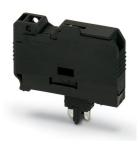
Fuse plug, Prior to replacing the cartridge fuse, disconnect the fuse connector from the basic terminal block., nom. voltage: 500 V, nominal current: 10 A, connection method: Plug-in connection, fuse type:  $G / 6,3 \times 32$ , color: black
