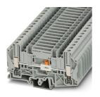
Disconnect terminal block, with spring support, nom. voltage: 1000 V, nominal current: 41 A, connection method: Screw connection, 1 level, Rated cross section: 6 mm<sup>2</sup>, cross section: 0.2 mm<sup>2</sup> - 10 mm<sup>2</sup>, mounting type: NS 35/7,5, NS 35/15, NS 32, color: gray
