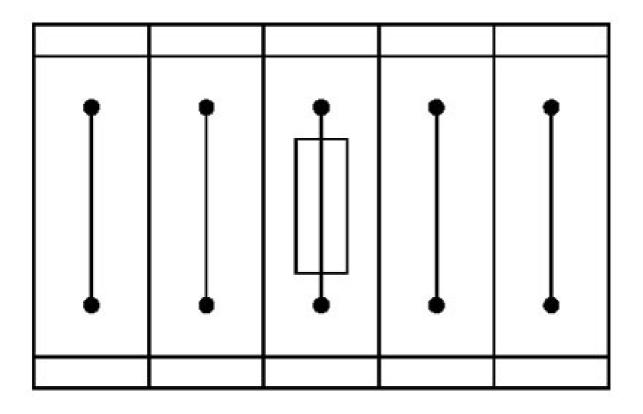
Fuse terminal block in single arrangement,
