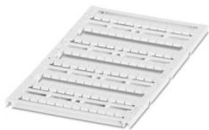
Marker for terminal blocks, Sheet, white, unlabeled, can be labeled with: BLUEMARK ID COLOR, BLUEMARK ID, BLUEMARK CLED, PLOTMARK, CMS-P1-PLOTTER, mounting type: snapped, for terminal block width: 5.2 mm, lettering field size: 4.6 x 5.1 mm, Number of individual labels: 96
