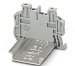
Quick mounting end clamp for NS 35/7,5 DIN rail or NS 35/15 DIN rail, with marking option, with parking option for FBS...5, FBS...6, KSS 5, KSS 6, width: 5.15 mm, color: gray
