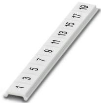
Zack Marker strip, flat, Strip, white, labeled, printed horizontally: Odd numbers 1 - 19, 21 - 39, etc. up to 81 - 99, mounting type: snapped, for terminal block width: 5 mm, lettering field size: 5.15 x 5.15 mm, Number of individual labels: 10
