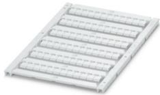
Marker for terminal blocks, Sheet, white, unlabeled, can be labeled with: TOPMARK NEO, TOPMARK LASER, BLUEMARK ID COLOR, BLUEMARK ID, BLUEMARK CLED, THERMOMARK PRIME, THERMOMARK CARD 2.0, THERMOMARK CARD, mounting type: snapped, for terminal block width: 5.2 mm, lettering field size: 4.4 x 4.7 mm, Number of individual labels: 72
