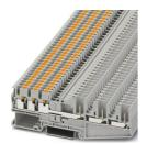
Feed-through terminal block, nom. voltage: 500 V, nominal current: 24 A, number of connections: 6, connection method: Push-in / plug connection, 1st, 2nd and 3rd level, Rated cross section: 2.5 mm<sup>2</sup>, cross section: 0.14 mm<sup>2</sup> - 4 mm<sup>2</sup>, mounting type: NS 35/7,5, NS 35/15, color: gray
