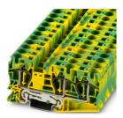
Ground terminal, number of connections: 3, connection method: Spring-cage connection, Rated cross section:  $16~\text{mm}^2$ , cross section:  $0.2~\text{mm}^2$  -  $25~\text{mm}^2$ , mounting type: NS 35/15, NS 35/7,5, color: green-yellow
