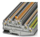
Disconnect terminal block, nom. voltage: 500 V, nominal current: 30 A, connection method: Push-in connection, Rated cross section: 4 mm $^2$ , cross section: 0.2 mm $^2$  - 6 mm $^2$ , connection method: Push-in connection, Rated cross section: 4 mm $^2$ , cross section: 0.2 mm $^2$  - 6 mm $^2$ , mounting: NS 35/7,5, NS 35/15, color: gray
