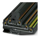
Fuse modular terminal block, fuse type: Glass / ceramics / ..., fuse type: G / 5 x 20, nom. voltage: 24 V, nominal current: 6.3 A, connection method: Push-in connection, Rated cross section: 4  $\text{mm}^2$ , cross section: 0.2  $\text{mm}^2$ - 6  $\text{mm}^2$ , connection method: Push-in connection, cross section: 0. 2  $\text{mm}^2$ - 6  $\text{mm}^2$ , mounting type: NS 35/7,5, NS 35/15, color: black
