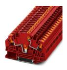
Test disconnect terminal block, nom. voltage: 1000 V, nominal current: 30 A, connection method: Push-in connection, Rated cross section:  $6 \text{ mm}^2$ , cross section:  $0.5 \text{ mm}^2$  -  $6 \text{ mm}^2$ , color: red
