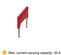
Plug-in bridge, pitch: 8.2 mm, number of positions: 5, pin assignment: 1,5, color: red
