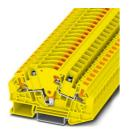
Test disconnect terminal block, nom. voltage: 1000 V, nominal current: 30 A, connection method: Push-in connection, Rated cross section: 6 mm², cross section: 0.5 mm² - 6 mm², color: yellow
