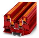
Feed-through terminal block, nom. voltage: 1000 V, nominal current: 41 A, number of connections: 4, number of positions: 1, connection method: Push-in connection, Rated cross section: 6 mm², cross section: 0.5 mm² - 10 mm², mounting type: NS 35/7,5, NS 35/15, color: red
