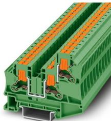
Feed-through terminal block, nom. voltage: 1000 V, nominal current: 41 A, number of connections: 3, number of positions: 1, connection method: Push-in connection, Rated cross section: 6 mm<sup>2</sup>, cross section: 0.5 mm<sup>2</sup> - 10 mm<sup>2</sup>, mounting type: NS 35/7,5, NS 35/15, color: green
