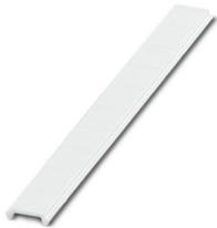
Zack Marker strip, flat, Strip, can be ordered: Strip, white, labeled according to customer specifications, mounting type: snap into flat marker groove, for terminal block width: 6.2 mm, lettering field size: 5.15 x 6.15 mm, Number of individual labels: 10
