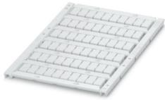
Marker for terminal blocks, Sheet, white, unlabeled, can be labeled with: TOPMARK NEO, TOPMARK LASER, BLUEMARK ID COLOR, BLUEMARK ID, BLUEMARK CLED, THERMOMARK PRIME, THERMOMARK CARD 2.0, THERMOMARK CARD, mounting type: snapped, for terminal block width: 6.2 mm, lettering field size: 5.6 x 10.5 mm, Number of individual labels: 60
