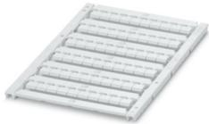
Marker for terminal blocks, can be ordered: by sheet, white, labeled according to customer specifications, mounting type: snap into flat marker groove, for terminal block width: 6.2 mm, lettering field size: 5.4 x 4.7 mm, Number of individual labels: 60
