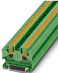
Feed-through terminal block, nom. voltage: 1000 V, nominal current: 32 A, number of connections: 2, connection method: Push-in connection, Rated cross section: 4 mm<sup>2</sup>, cross section: 0.2 mm<sup>2</sup> - 6 mm<sup>2</sup>, mounting type: NS 35/7,5, NS 35/15, color: green
