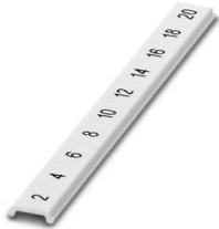
Zack Marker strip, flat, Strip, white, labeled, printed horizontally: consecutive even numbers 2 ... 20, 22 ... 40, etc. up to 82 ... 100, mounting type: snapped, for terminal block width: 6.2 mm, lettering field size: 5.15 x 6.15 mm, Number of individual labels: 10
