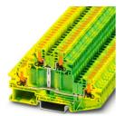
Protective conductor double-level terminal block, number of connections: 4, connection method: Push-in connection, 1st and 2nd level, Rated cross section: 4 mm², cross section: 0.2 mm² - 6 mm², mounting type: NS 35/7,5, NS 35/15, color: green/yellow
