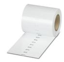
Marker for terminal blocks, can be ordered: by line, white, labeled according to customer specifications, mounting type: snap into universal marker groove, snap into flat marker groove, for terminal block width: 6.2 mm, lettering field size: 6. 35 x 6 15 mm
