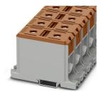
High-current terminal block, nom. voltage: 1000 V, nominal current: 290 A, number of connections: 2, number of positions: 1, connection method: Screw connection, Rated cross section: 150 mm<sup>2</sup>, cross section: 35 mm<sup>2</sup> - 150 mm<sup>2</sup>, Rated cross section: 150 mm<sup>2</sup>, cross section: 35 mm<sup>2</sup> - 150 mm<sup>2</sup>, mounting type: NS 35/15, NS 35/7,5, color: brown
