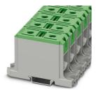
High-current terminal block, nom. voltage: 1000 V, nominal current: 220 A, number of connections: 2, number of positions: 1, connection method: Screw connection, Rated cross section: 95 mm<sup>2</sup>, cross section: 16 mm<sup>2</sup> - 95 mm<sup>2</sup>, Rated cross section: 95 mm<sup>2</sup>, cross section: 16 mm<sup>2</sup> - 95 mm<sup>2</sup>, mounting type: NS 35/15, NS 35/7,5, color: green
