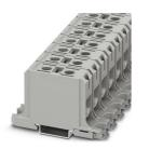
High-current terminal block, nom. voltage: 1000 V, nominal current: 145 A, number of connections: 2, number of positions: 1, connection method: Screw connection, Rated cross section: 50 mm<sup>2</sup>, cross section: 6 mm<sup>2</sup> - 50 mm<sup>2</sup>, Rated cross section: 50 mm<sup>2</sup>, cross section: 4 mm<sup>2</sup> - 50 mm<sup>2</sup>, mounting type: NS 35/15, NS 35/7,5, color: gray
