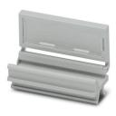
Group marking label, snaps onto terminal center for screw, spring-cage and quick connection terminal blocks, labeled with ESL 26x6 mm or EST 25x6 mm, in the foot part with Zack marker strip, length: 29 mm
