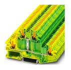
Protective conductor double-level terminal block, number of connections: 4, connection method: Push-in connection, 1st and 2nd level, Rated cross section: 2.5 mm<sup>2</sup>, cross section: 0.14 mm<sup>2</sup> - 4 mm<sup>2</sup>, mounting type: NS 35/7,5, NS 35/15, color: green-yellow
