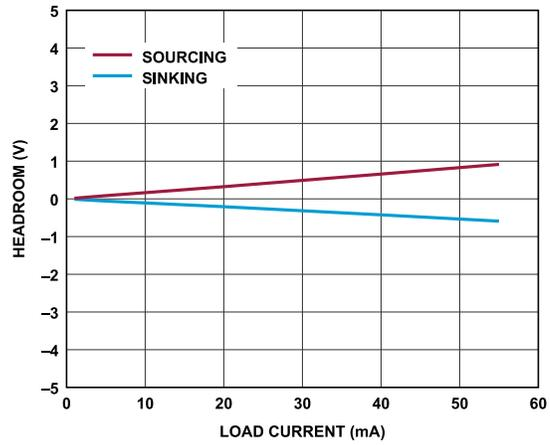
Figure 44.  $V_{x^+}/V^-$  Unipolar Headroom vs. Output Load Current
