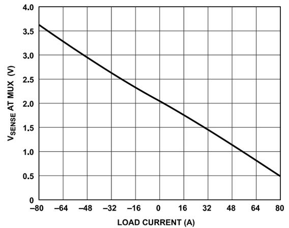
Figure 21.  $V_{SENSE}$  at MUX vs. Load Current
