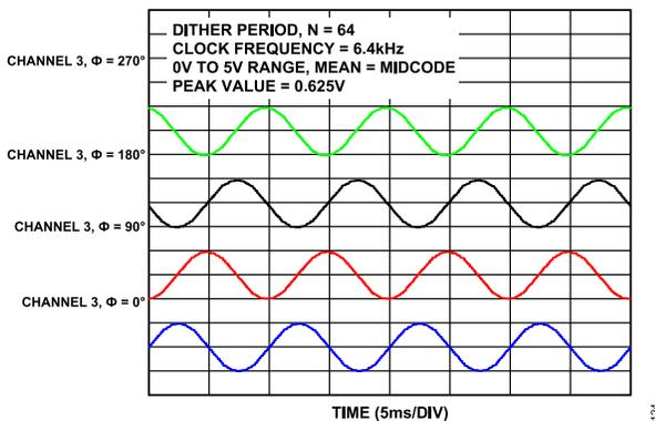
Figure 25. Sinusoidal Dither for Various Phase Settings
