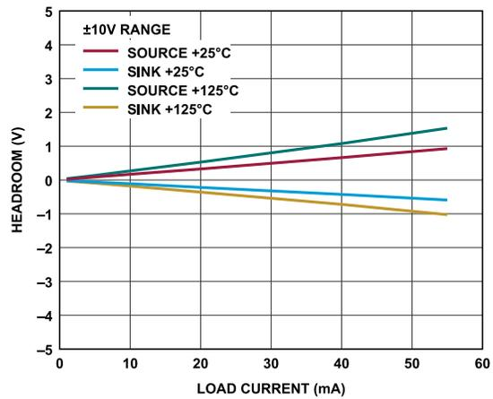
Figure 45.  $V_{x^+}/V^-$  Bipolar Headroom vs. Output Load Current
