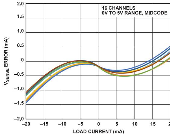
Figure 46.  $V_{SENSE}$  Error vs. Load Current from Equation 5
