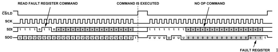
Figure 50. Typical Read Command Sequence for 24-Bit Words
