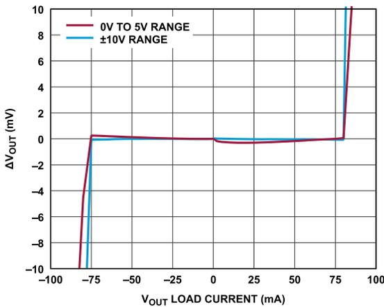
Figure 19.  $\Delta V_{OUT}$  vs.  $V_{OUT}$  Load Current
