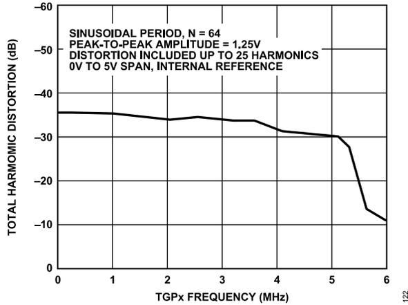
Figure 23. Total Harmonic Distortion vs. TGPx Frequency
