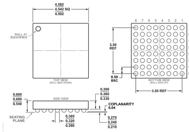
**Figure 62. 64-Ball Wafer Level Chip Package [WLCSP]
