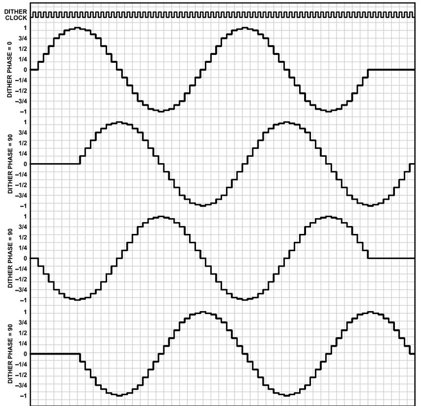
Figure 57. Sinusoidal Waveforms for Various Values of  $\Phi_0$
