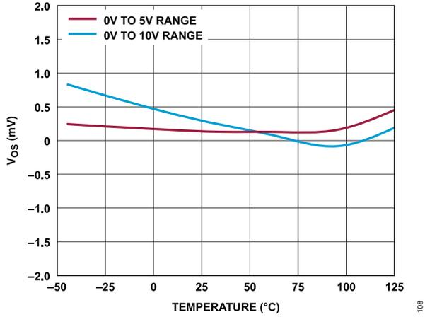
Figure 9. Unipolar Offset Error ( $V_{OS}$ ) vs. Temperature
