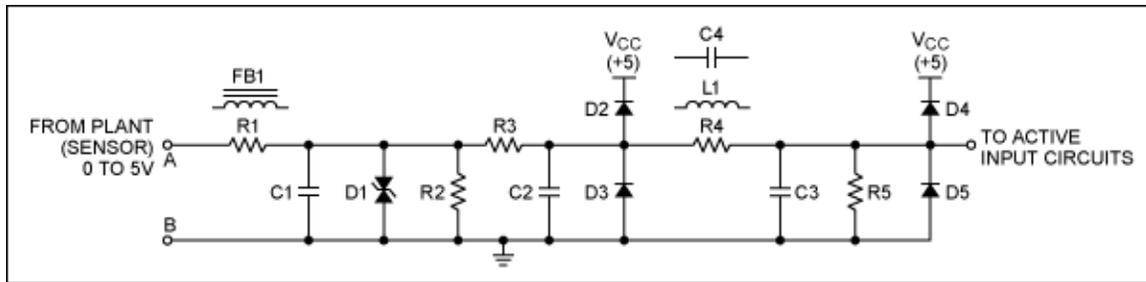
Figure 6. An inventory of suggested discrete components which can protect against unwanted electrical vulnerabilities.
