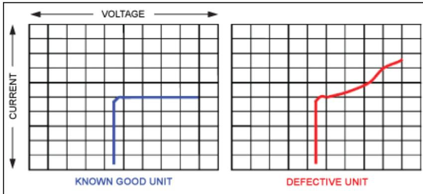
Figure 4. Semiconductor curve tracer plots for the circuit in Figure 3. Curve tracer current/div. is 50 $\mu$ A; voltage/div. is 1V.
