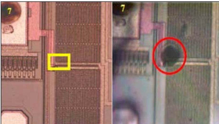
Figure 3. A circuit (left) under visible light shows no apparent damage from the lightning bolt. The same circuit (right) under a microscope shows a hot spot with damage.
