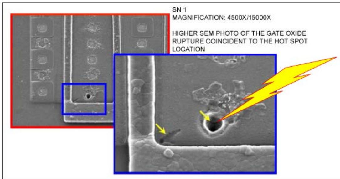
Figure 5. Scanning electron microscope photos of the circuit in Figure 3. The lightning bolt caused a hole in the gate oxide, which shorted the circuit.
