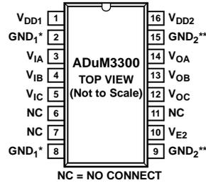
\*PIN 2 AND PIN 8 ARE INTERNALLY CONNECTED, AND CONNECTING BOTH TO GND<sub>1</sub> IS RECOMMENDED.
