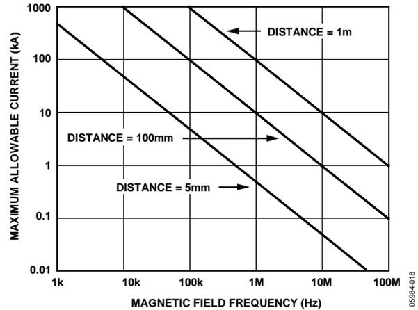
Figure 17. Maximum Allowable Current for Various Current-to-ADuM3300/ADuM3301 Spacings
