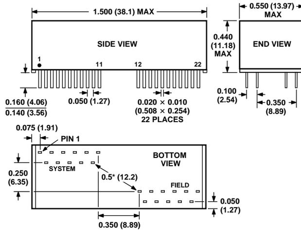
\* CREEPAGE PATH (SUBTRACT APPROXIMATELY 0.079 (2mm) FOR SOLDER PAD RADII ON PC BOARD. THIS SPACING SUPPORTS THE INTRINSICALLY SAFE RATING OF 750V. WAVE SOLDERING IS NOT RECOMMENDED.
