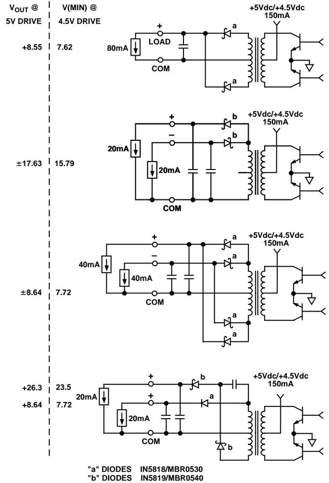
Figure 5. Field Side Power Supply Rectifier Examples
