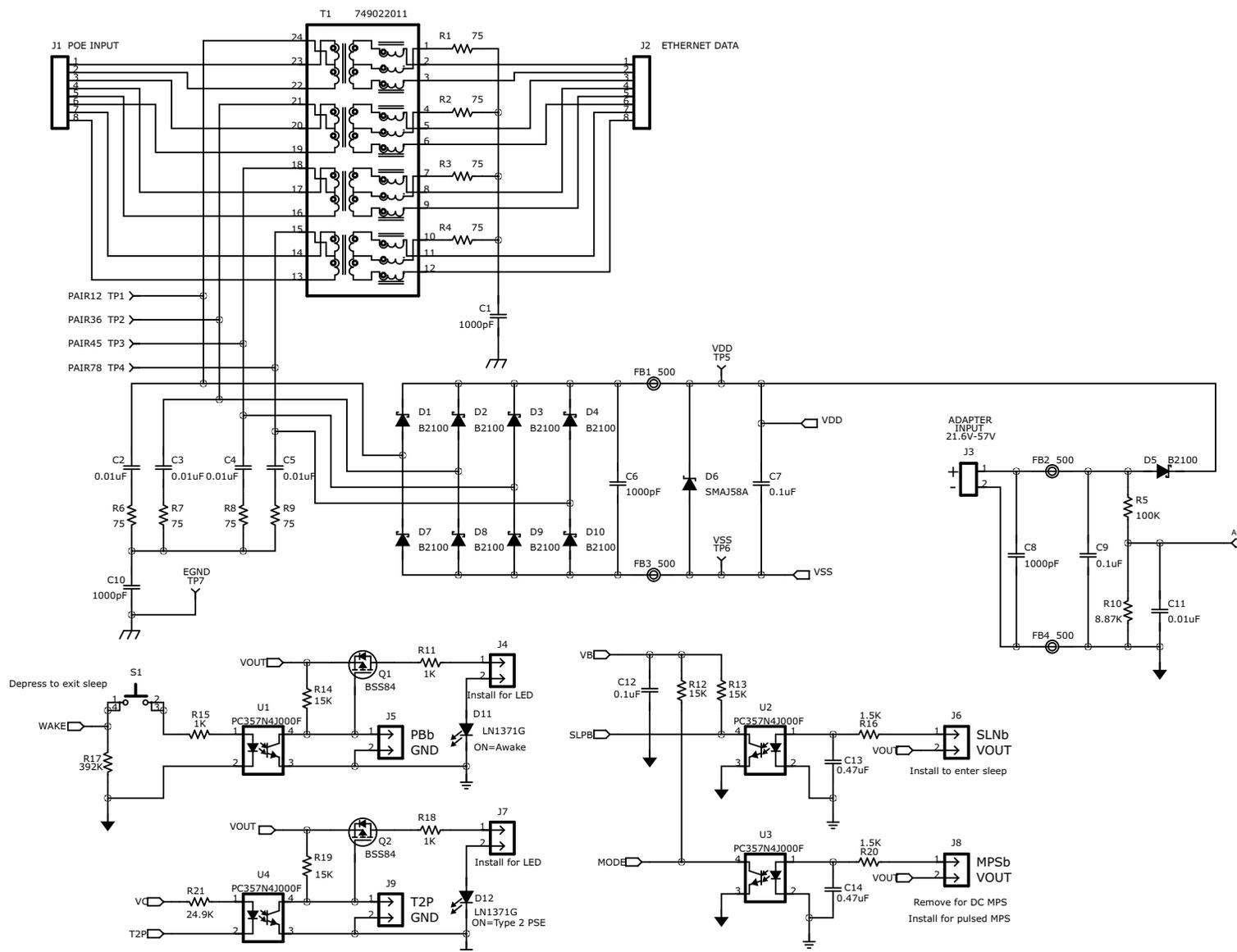
Figure 1. TPS23752EVM-145 Schematic
