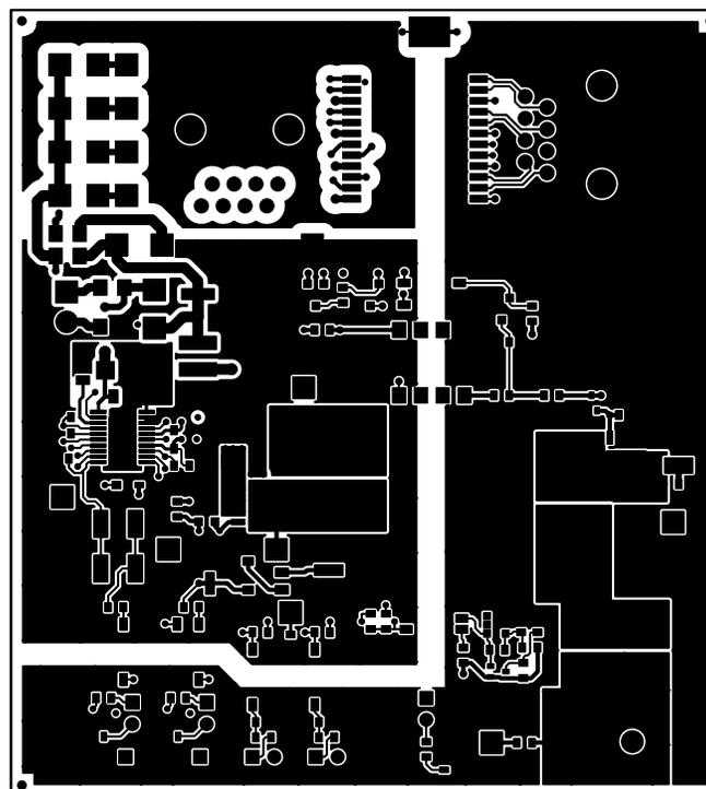
Figure 8. Top-Side Routing
