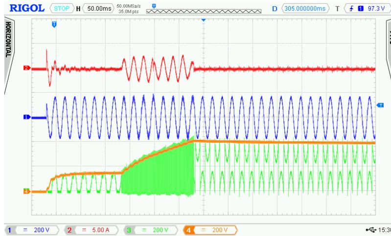
**Figure 4-7: No-load start-up at 115 V<sub>ac</sub> input. Channel 1(Blue): Input ac voltage (200 V/div); Channel 2(Red): Input ac current (5 A/div); Channel 3(Green): TP-PFC high frequency leg switch node voltage (200 V/div); Channel 4(Orange): Output voltage (200 V/div); time: 50 ms/div.**
