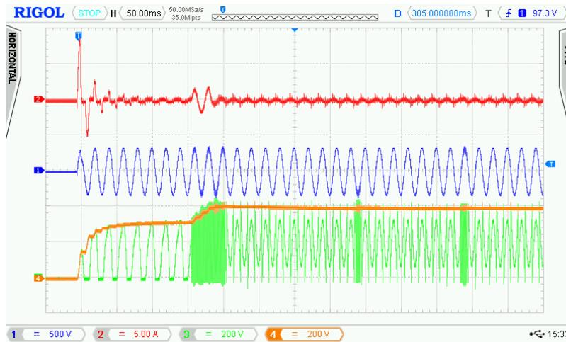
**Figure 4-8: No-load start-up at 230 V<sub>ac</sub> input. Channel 1(Blue): Input ac voltage (500 V/div); Channel 2(Red): Input ac current (5 A/div); Channel 3(Green): TP-PFC high frequency leg switch node voltage (200 V/div); Channel 4(Orange): Output voltage (200 V/div); time: 50 ms/div.**
