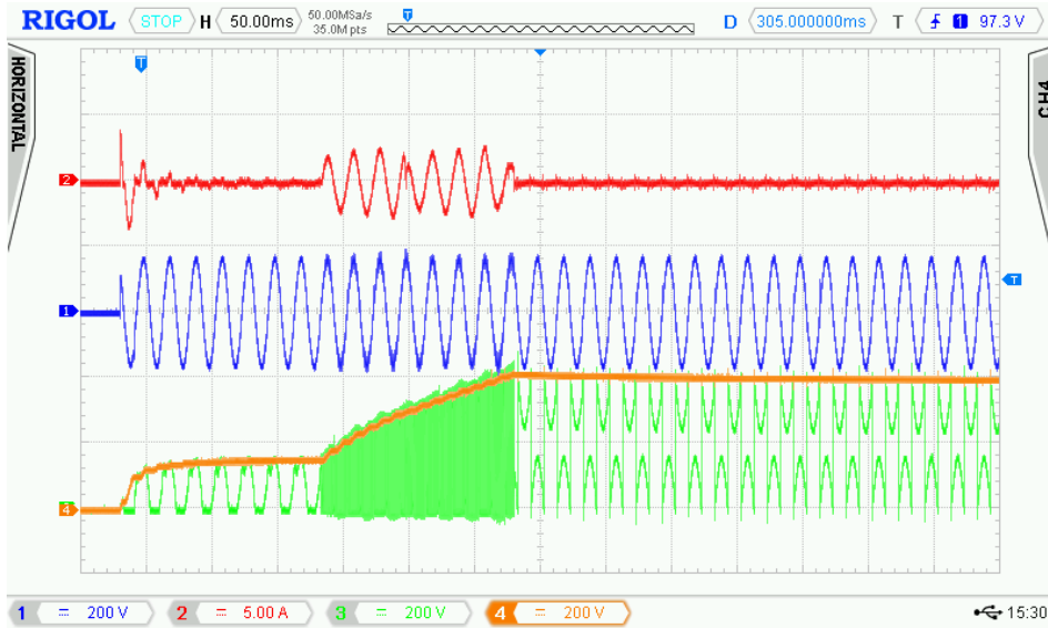
Figure 4-7: No-load start-up at 115 V ac input. Channel 1(Blue): Input ac voltage (200 V/div); Channel 2(Red): Input ac current (5 A/div); Channel 3(Green): TP-PFC high frequency leg switch node voltage (200 V/div); Channel 4(Orange): Output voltage (200 V/div); time: 50 ms/div.
