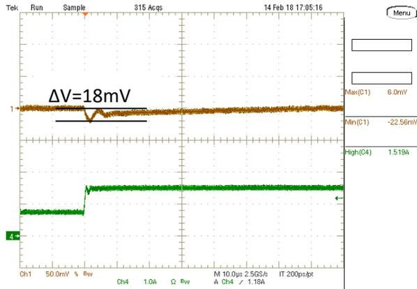
Step Load Transient Response ( $V_{in}=5V$ ,  $V_{out4}=2.5V$ ,
