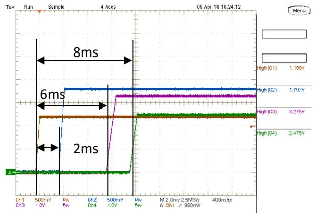
On/Off Enable Delay (Vin=5.0V, Iout=MAX)
