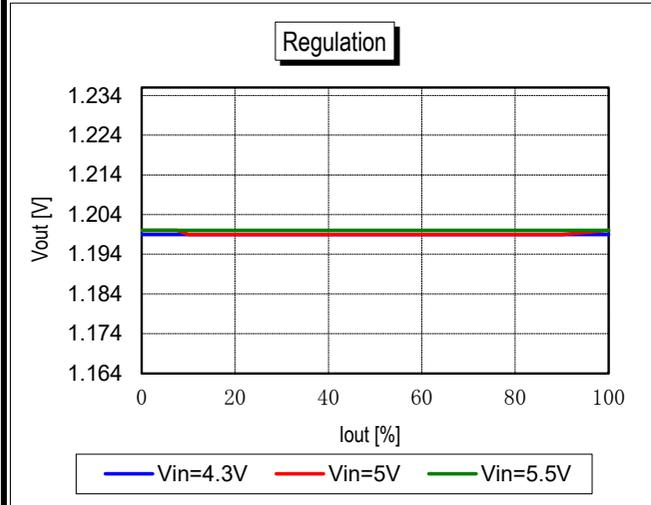
Vout2 vs. Line Voltage and Load Current @ +25degC.
