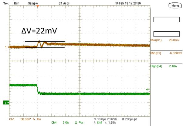
Step Load Transient Response ( $V_{in}=5V$ ,  $V_{out2}=1.8V$ ,
