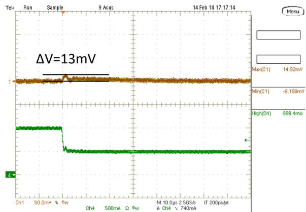
Step Load Transient Response ( $V_{in}=5V$ ,  $V_{out3}=3.3V$ ,
