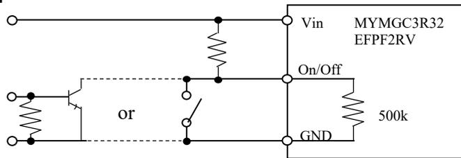
It is strongly recommended that on/off terminal should be used when you turn on/off this product. Characteristics may be affected by turning input voltage on/off. Please check product operation on your application with turning input voltage on/off.
