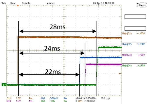
On/Off Enable Delay (Vin=5.0V, Iout=MAX)
