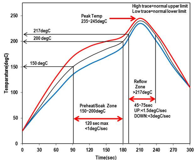
**CAUTION:** Do not reflow the converter as follows, because the converter may fall from the substrate during reflowing.
