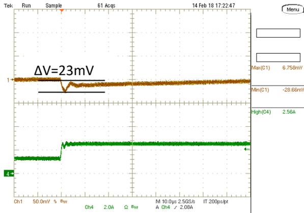
Step Load Transient Response ( $V_{in}=5V$ ,  $V_{out1}=1.2V$ ,
