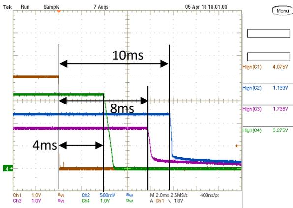
On/Off Enable Delay (Vin=5.0V, Iout=MAX)
