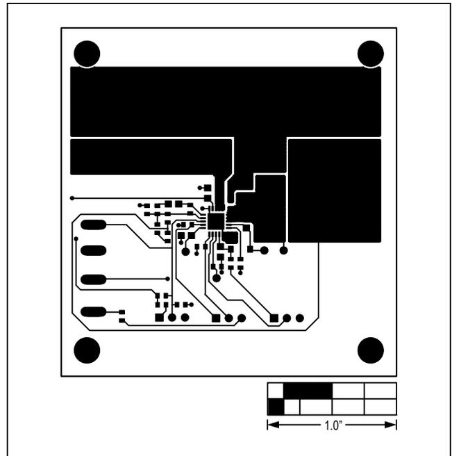
Figure 3. MAX15020 EV Kit PCB Layout—Component Side
