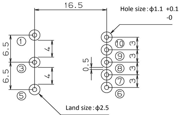
※ The round pulling out figure is a pin numbering.
