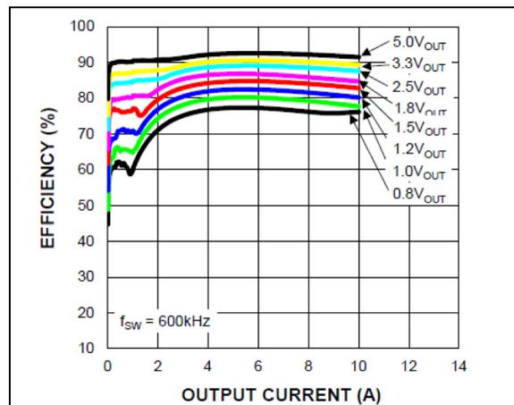
**FIGURE 2-12:** Efficiency ( $V_{IN} = 12V$ ) vs. Output Current (MIC45208-1).
