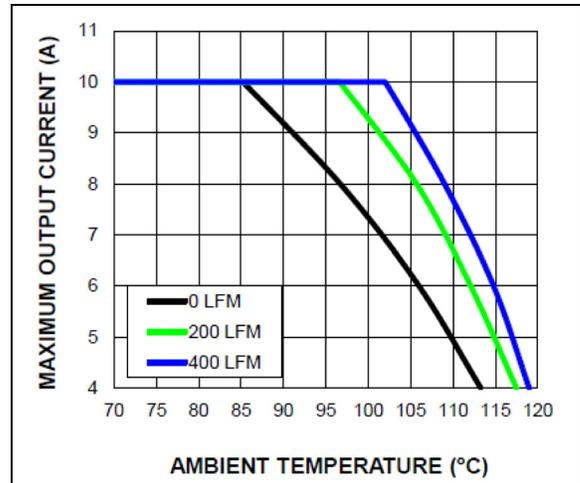
FIGURE 5-7: MIC45208 Power Derating vs. Airflow (12 V<sub>IN</sub> to 1.5 V<sub>OUT</sub>).
