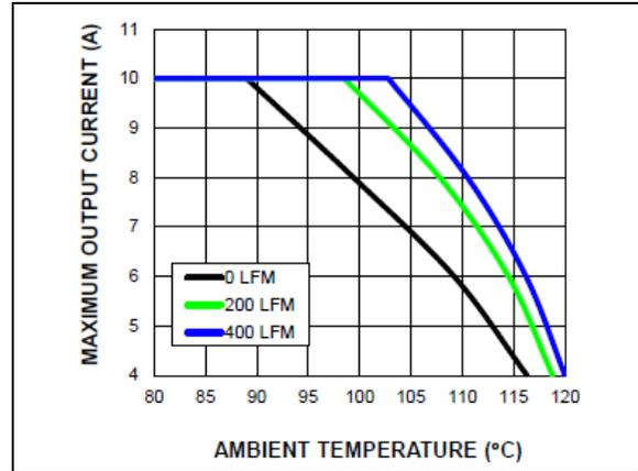
FIGURE 5-6: MIC45208 Power Derating vs. Airflow (5 V<sub>IN</sub> to 1.5 V<sub>OUT</sub>).
