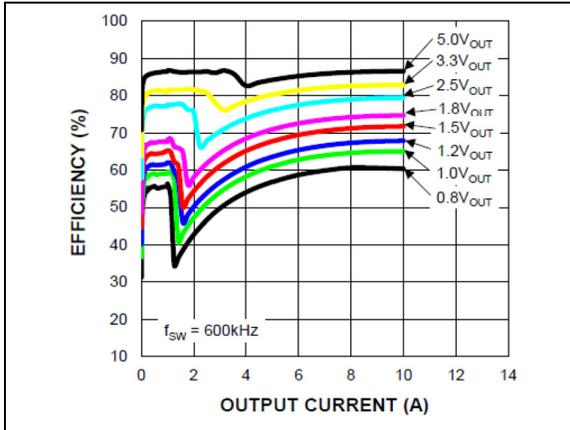
**FIGURE 2-13:** Efficiency ( $V_{IN} = 24V$ ) vs. Output Current (MIC45208-1).
