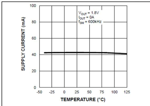
**FIGURE 2-2:**  $V_{IN}$  Operating Supply Current vs. Temperature (MIC45208-2).
