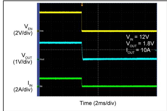
**FIGURE 2-25:** Enable Turn-Off Delay and Fall Time.
