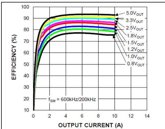
**FIGURE 2-15:** Efficiency ( $V_{IN} = 12V$ ) vs. Output Current (MIC45208-2).
