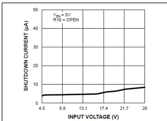
**FIGURE 2-3:**  $V_{IN}$  Shutdown Current vs. Input Voltage.
