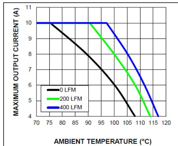
FIGURE 5-8: MIC45208 Power Derating vs. Airflow (12 V<sub>IN</sub> to 3.3 V<sub>OUT</sub>).
