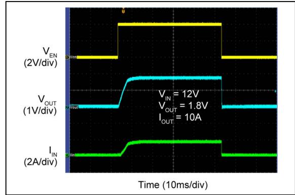
**FIGURE 2-27:** Enable Turn-On/Off.
