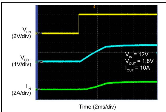
**FIGURE 2-24:** Enable Turn-On Delay and Rise Time.
