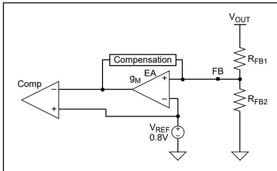
**FIGURE 4-1:** Output Voltage Sense via FB Pin.
