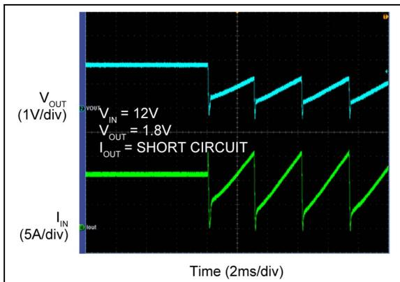
**FIGURE 2-30:** Short Circuit.
