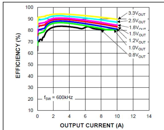
**FIGURE 2-11:** Efficiency ( $V_{IN} = 5V$ ) vs. Output Current (MIC45208-1).
