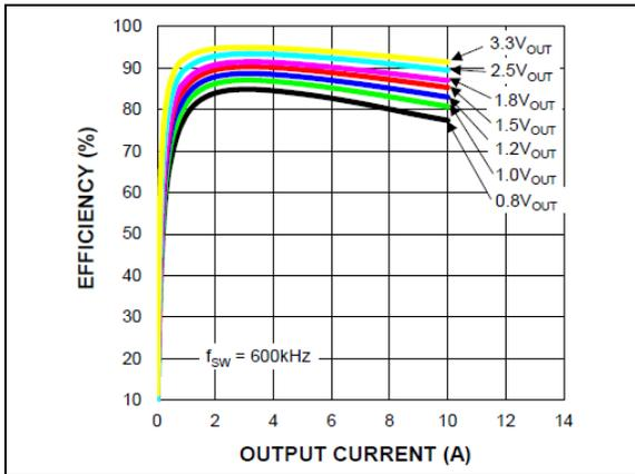
**FIGURE 2-14:** Efficiency ( $V_{IN} = 5V$ ) vs. Output Current (MIC45208-2).
