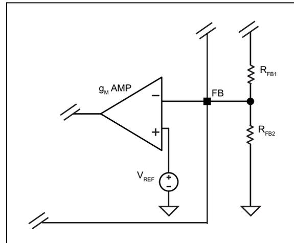
**FIGURE 5-3:** Voltage/Divider Configuration.
