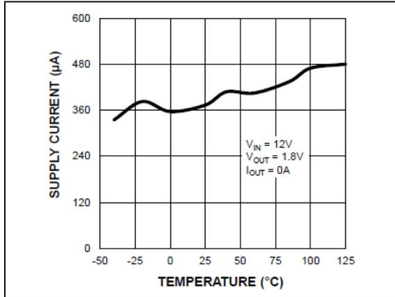
**FIGURE 2-1:**  $V_{IN}$  Operating Supply Current vs. Temperature (MIC45208-1).
