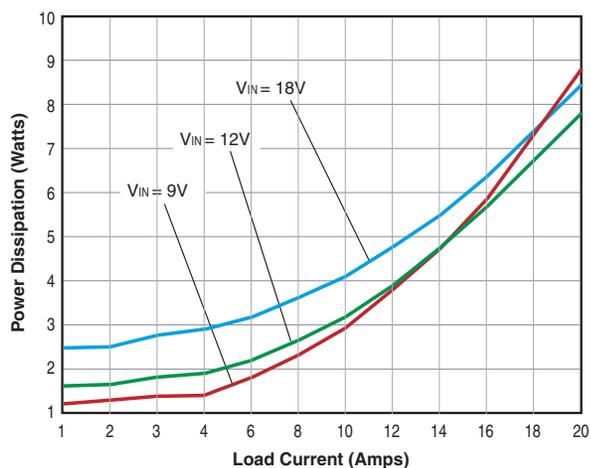
**ULE-3.3/20-D48 Power Dissipation vs. Load Current @ +25°C**
