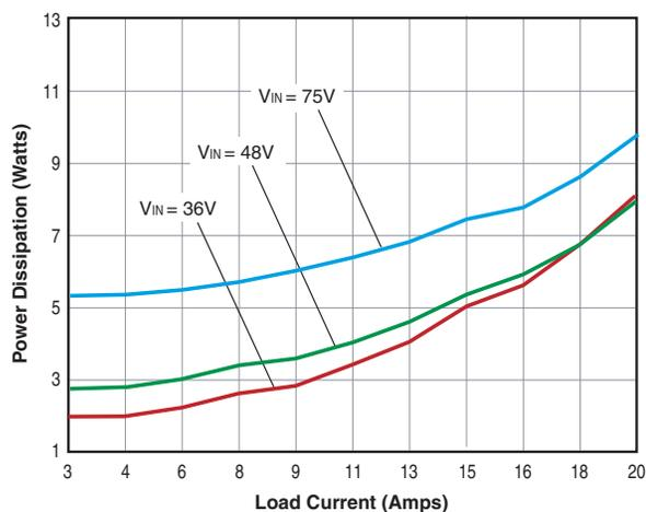
**ULE-5/10-D12 Power Dissipation vs. Load Current @ +25°C**
