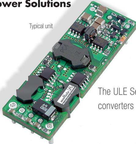
The ULE Series "Eighth-Brick" DC-DC Converters are high-current isolated power converters designed for use in high-density system boards.
