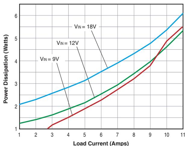
**ULE-5/12-D48 Power Dissipation vs. Load Current @ +25°C**
