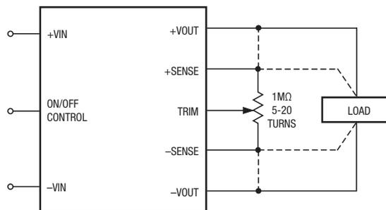
the converter's performance and are not recommended. Excessive voltage differences
