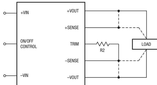
cause the overvoltage protection circuitry to activate (see Performance Specifications for overvoltage limits). Power derating is based on maximum output current and voltage at the converter's output pins. Use of trim and sense functions can cause output voltages to increase, thereby increasing output power beyond the converter's specified rating or cause output voltages to climb into the output overvoltage region. Therefore:
