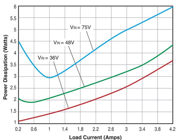
ULE-24/3-D48 Power Dissipation vs. Load Current @ +25°C
