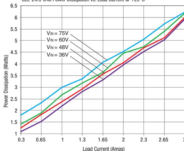
ULE-48/1.25-D48 Power Dissipation vs. Load Current @ +25°C
