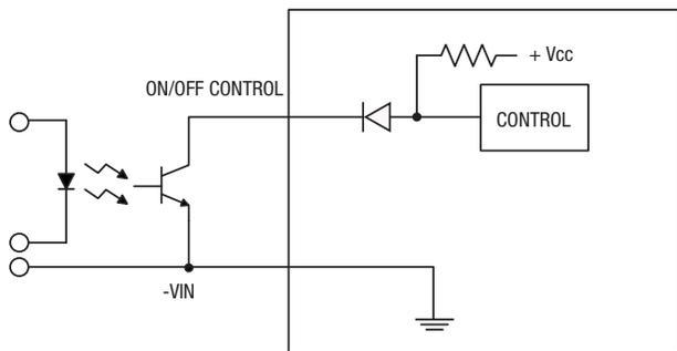
should be able to sink appropriate current (see Performance Specs) when activated and withstand appropriate voltage when deactivated. Applying an external voltage to the On/Off Control when no input power is applied to the converter can cause permanent damage to the converter.
