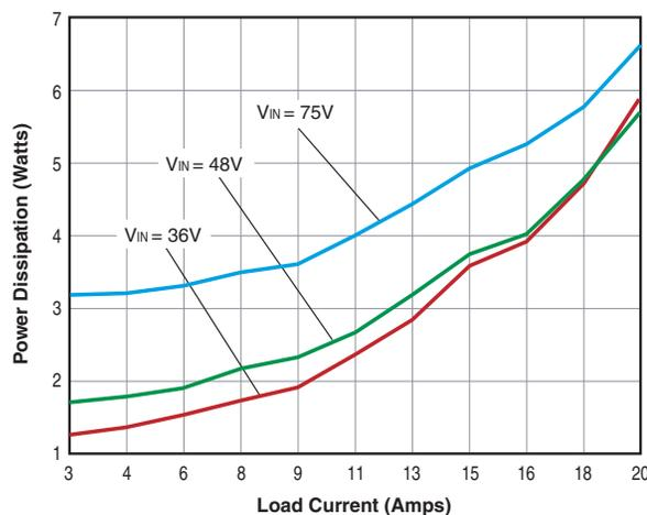
ULE-2.5/20-D48 Power Dissipation vs. Load Current @ +25°C
