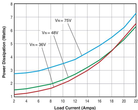
ULE-1.8/20-D48 Power Dissipation vs. Load Current @ +25°C
