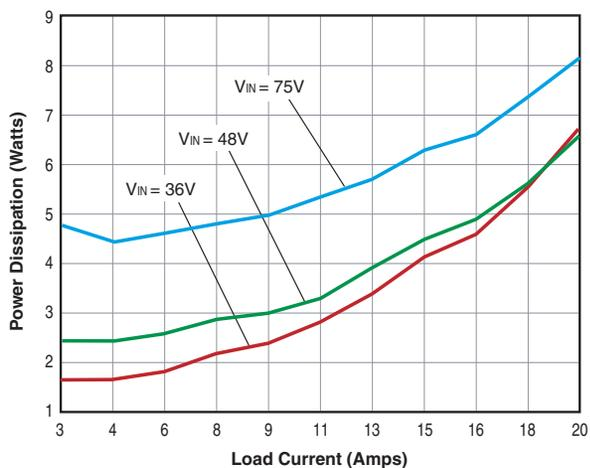
ULE-3.3/20-D24 Power Dissipation vs. Load Current @ +25°C
