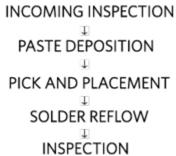
*Figure 3. Recommended uSLIC assembly process.*
